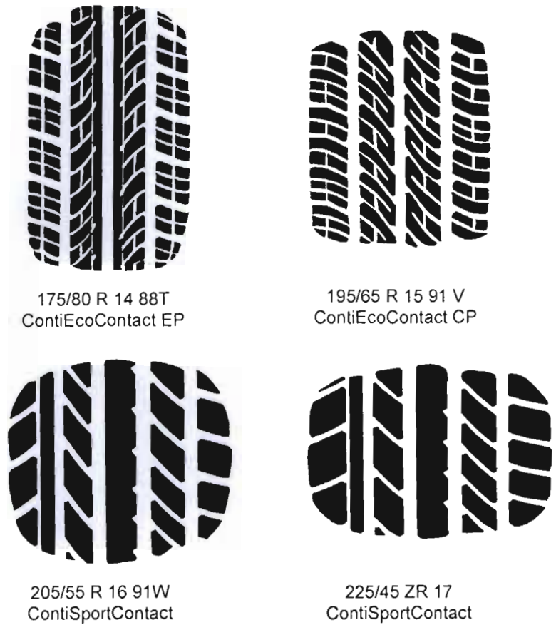
Fig. 2.9 If they have the same outside diameter and load capacity the four tyre sizes used on medium-sized passenger cars are interchangeable. The series 65, 55 and 45 wide tyres each allow a 1" larger rim (and therefore larger brake discs). The different widths and lengths of the tyre contact patch, known as 'tyre print', are clearly shown (Fig. 3.119), as are the different designs of the standard road profile and the asymmetric design of the sports profile (see also Section 2.2.10). The 65 series is intended for commercial vehicles, and the 60, 55 and 45 series for sports cars. (Illustration: Continental; see also Fig. 2.19.)
