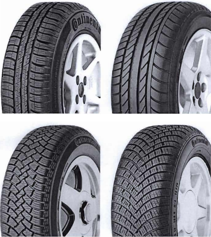
Fig. 2.19 Designs of Continental tyre. (Top) Summer tyre (tyre foot prints see Fig. 2.9) EcoContact EP (size 185/65 R14T) and Sport Contact (size 205/55 R16W). (Below) Winter tyre WinterContact TS760 (size 185/65 R14T) and WinterContact TS770 (size 235/60 R16H).
